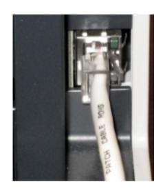
After inserting the network cable into the printer's NIC connector, insert the other end of the network cable into a network data drop in the wall nearest the printer. Network data drops may be identified -in most cases- by their orange color.
