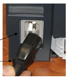
Correctly inserted AC power cord (right).
