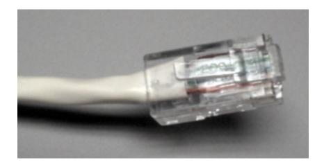
Good connector snap tab in place and undamaged.
