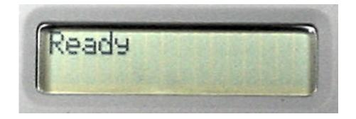
7. Wait one to two minutes and then depress the 'OK' button on the front panel two (2) times so the status display reads 'Reports Demo Page'.
